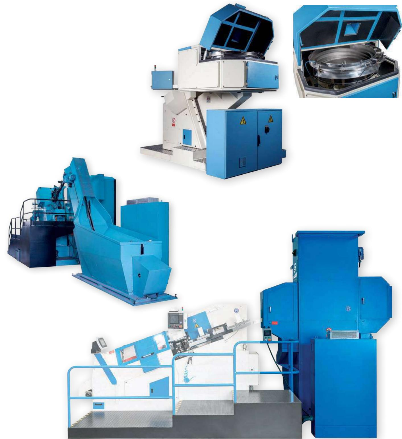
**Vertical feeding with hopper. The hopper consists of a folding ramp commanded by a load detector that assures a constant feeding.**
